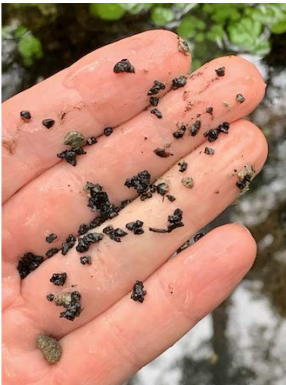
Rubber crumb found at a stormwater outlet below a synthetic turf sports field with rubber crumb infill
