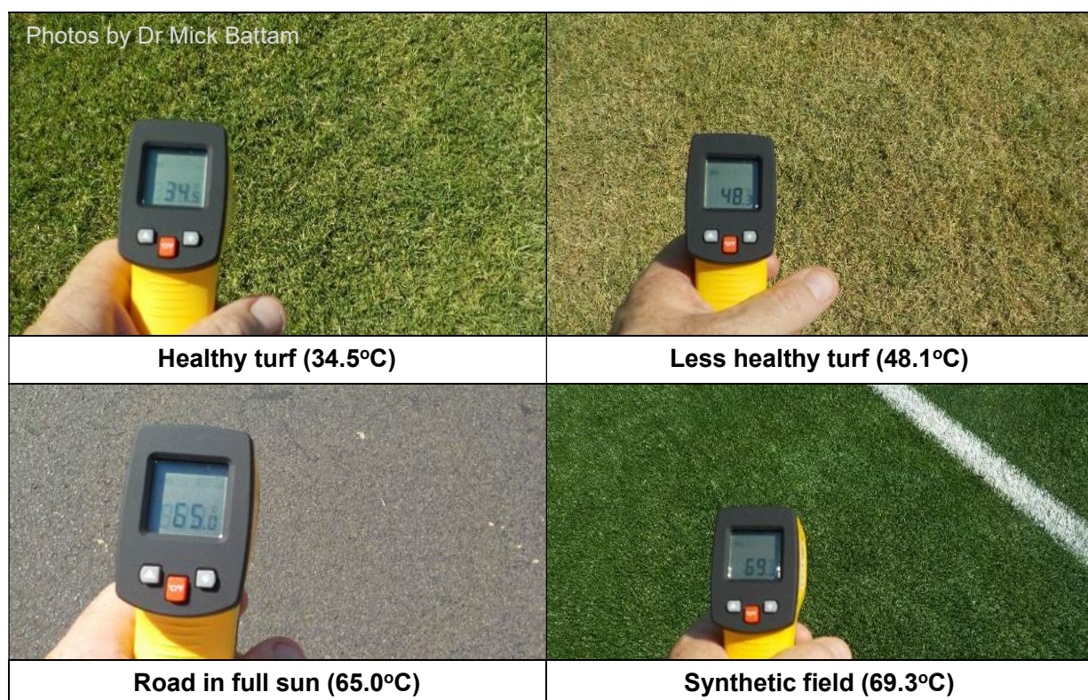
Figure 1.1: In addition to removing carbon dioxide from the atmosphere, natural turf can play a key role in combating urban heat islands as these temperatures taken on a 38°C day demonstrate.
