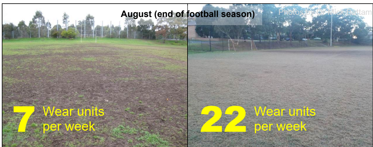
Figure 6.1: Two sporting fields about 7 km apart that have very different carrying capacities. The more intensely used field was built according to best practice principles and easily handles much higher levels of wear whilst requiring no patching, with the poorly built field struggling to handle low levels of wear. Photos taken at the end of football season when fields are at their worst.
