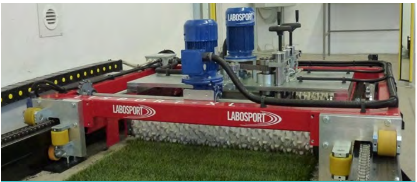
LisportXL durability testing machine (Labosport)
