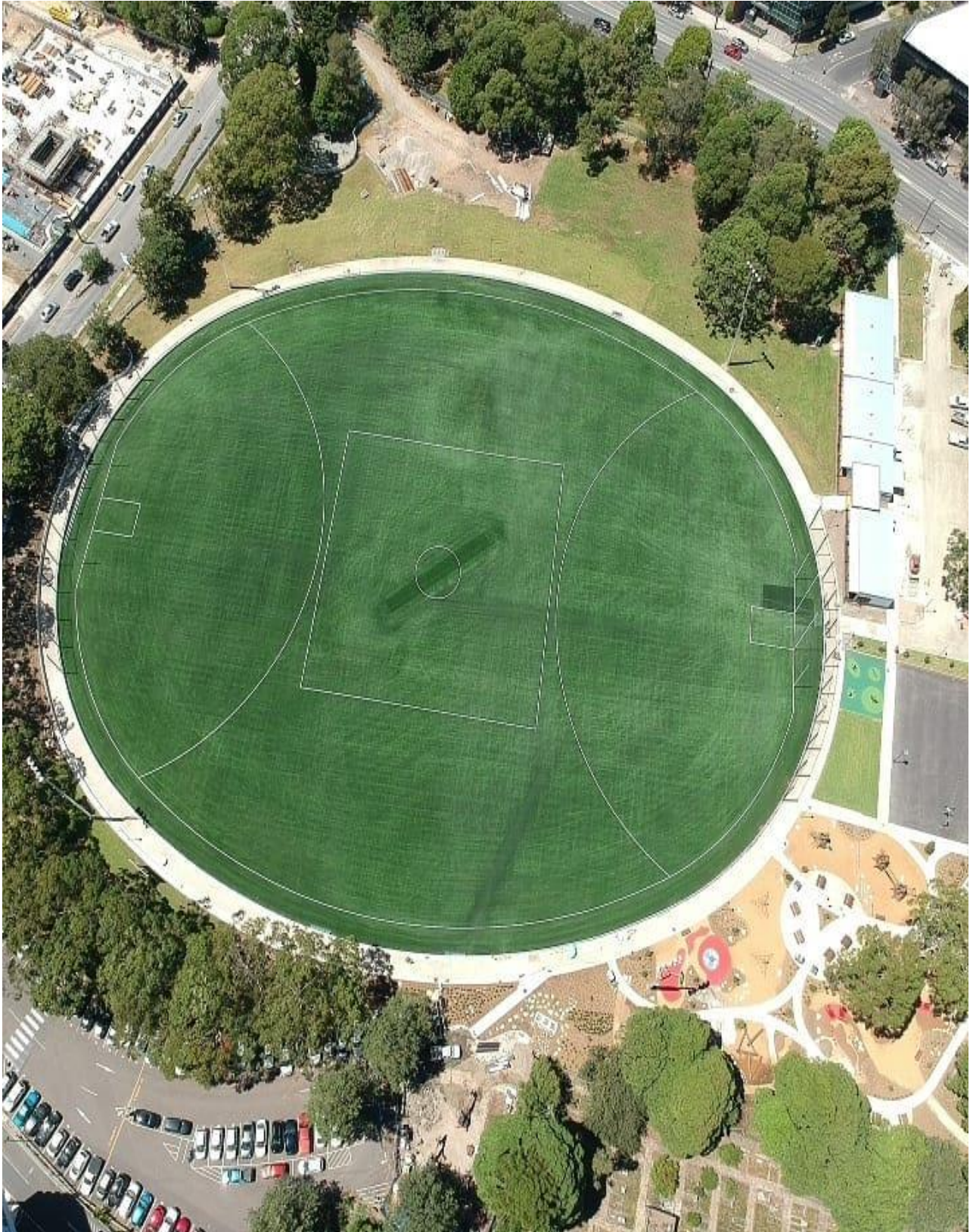
Gore Hill Oval, providing sustainability to community use as the natural turf field could not cope with the usage and the continued flooding (source: Willoughby City Council)
