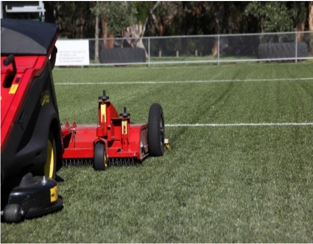
Photo 28: Tines being used to decompact infill and redistribute infill
