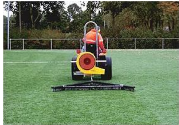
Photo 24: Least impact on Ball Roll was found on the Triangular Brush
