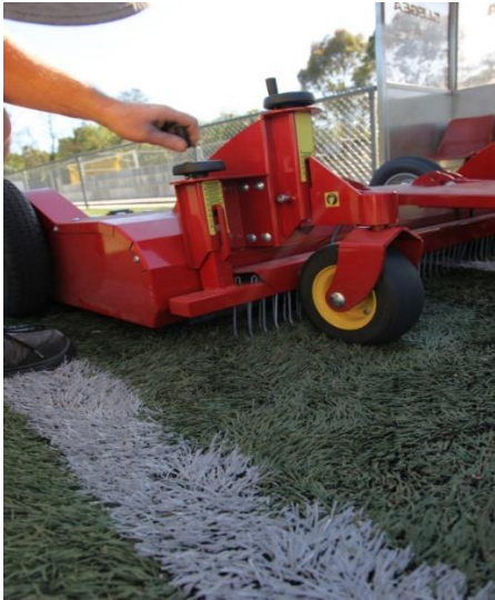
Photo 25: Setting the tines length to decompact a flat grass surface
