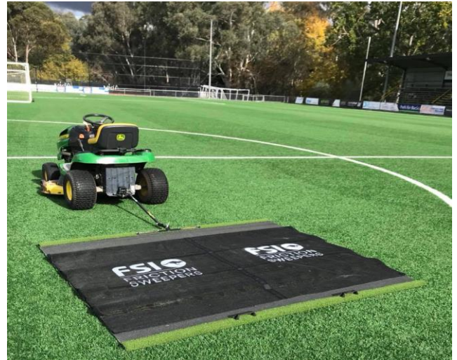
Photo 29: Friction Sweeper – Soft grass covered under-surface (source: Friction Sweepers International)
