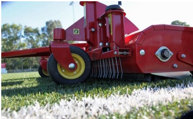
Photo 33: Modern machine providing height options for the tines to be used into the turf by an experienced operator
