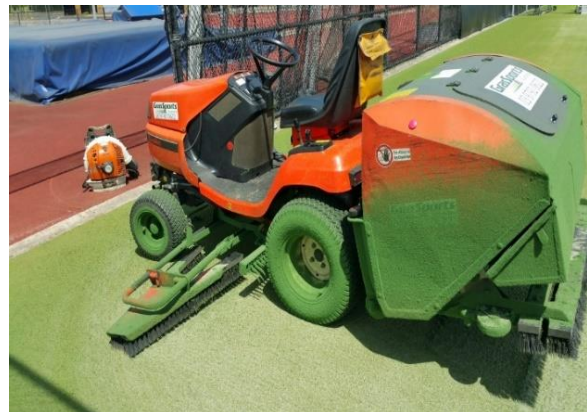
Photo 35: The yarn has been exposed to UV and the tips are breaking down and covering the maintenance machine
