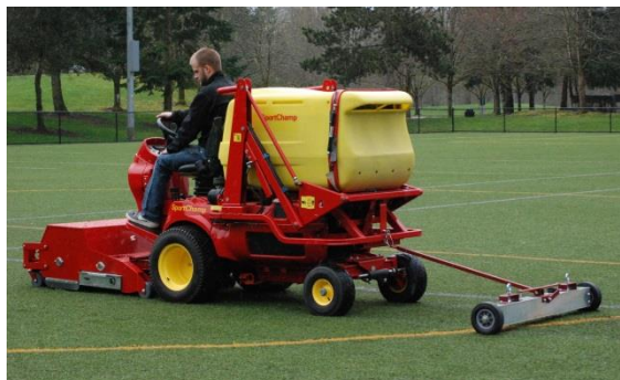
Photo 36: Machinery including the metal magnet at rear
