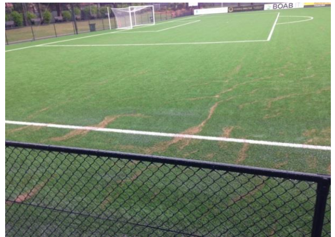
Photo 7: Organic infill displaced after rain, needs to be brushed to redistribute infill by using specialist machinery that can collect it and redistribute it accordingly (source: Smart Connection Consultancy)
