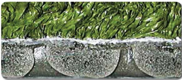
1st Generation Artificial Grass © Loughborough University; www.sportsturf.lboro.ac.uk • 10 – 12 mm fibre length, integral shock pad developed 1960s, nylon, unfilled, hard, abrasive • Used for hockey at the 1976 Montreal Olympics
