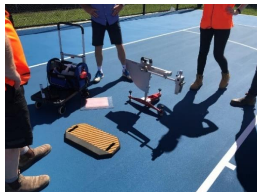
Photo 35: Testing apparatus for slip resistance
