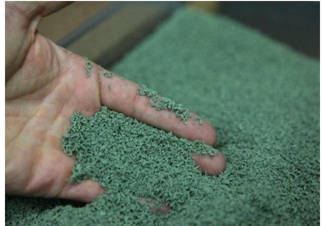
Photo 25: EPDM infill (source: Smart Connection Consultancy)
