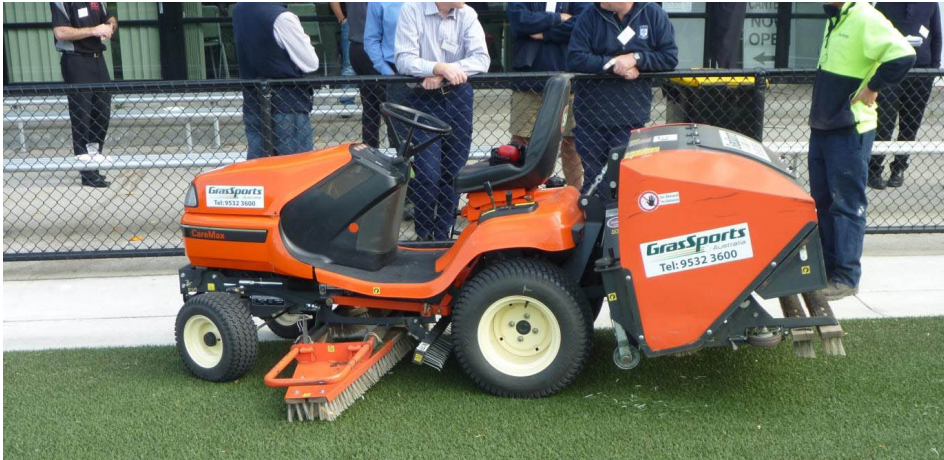
Figure 2: Ride on grooming and cleaning machine with petrol engine used to maintain synthetic turf.
