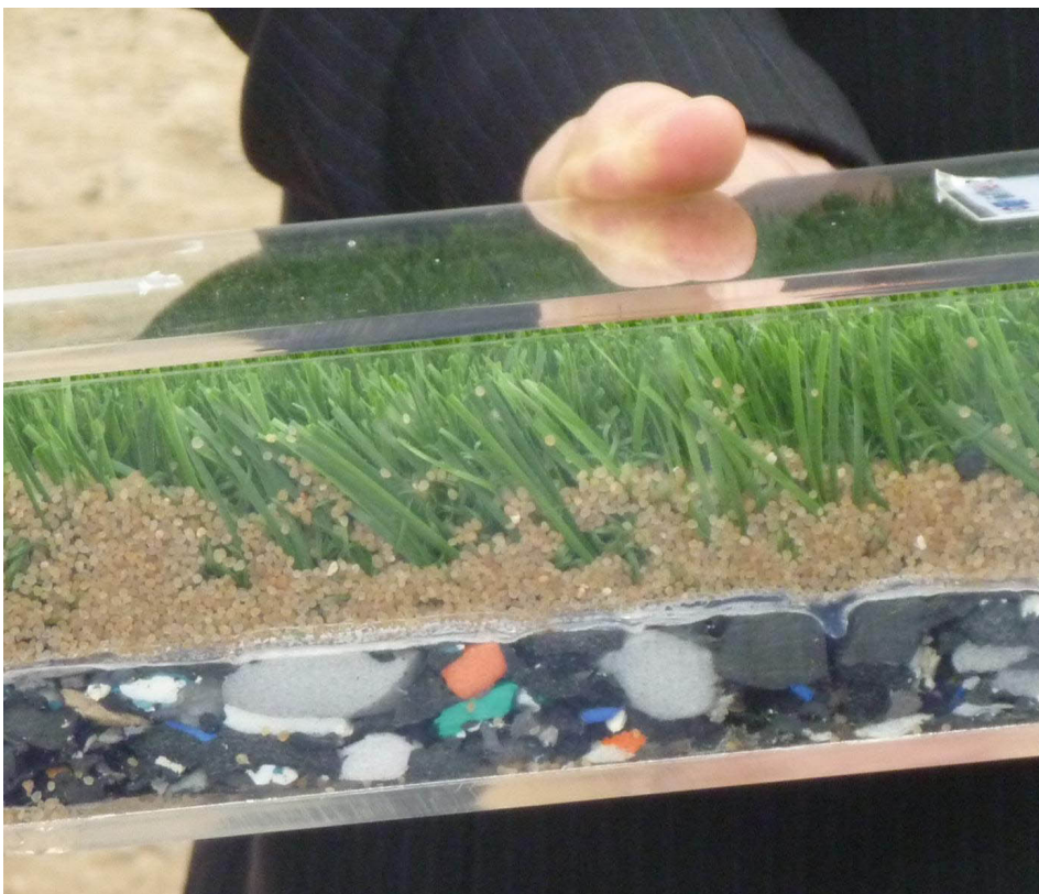
Figure 4: Rounded sand being used as the turf infill in place of rubber granules
