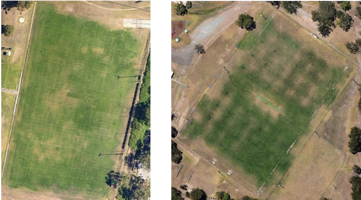
Figure 11.1: Two aerial images showing the impact of uneven water distribution on turf performance (Nearmaps images).
