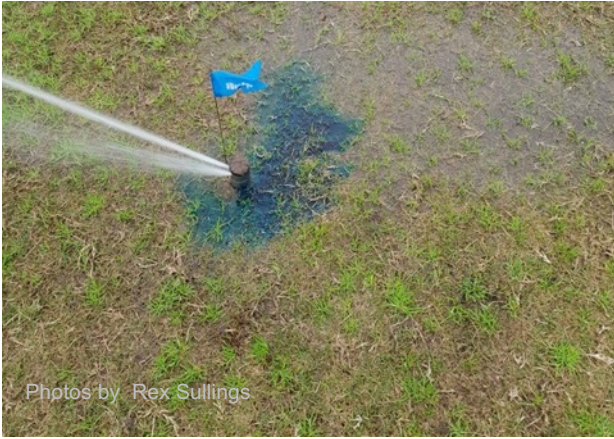
Examples of sprinklers leaking from riser seal or from below the sprinkler.
