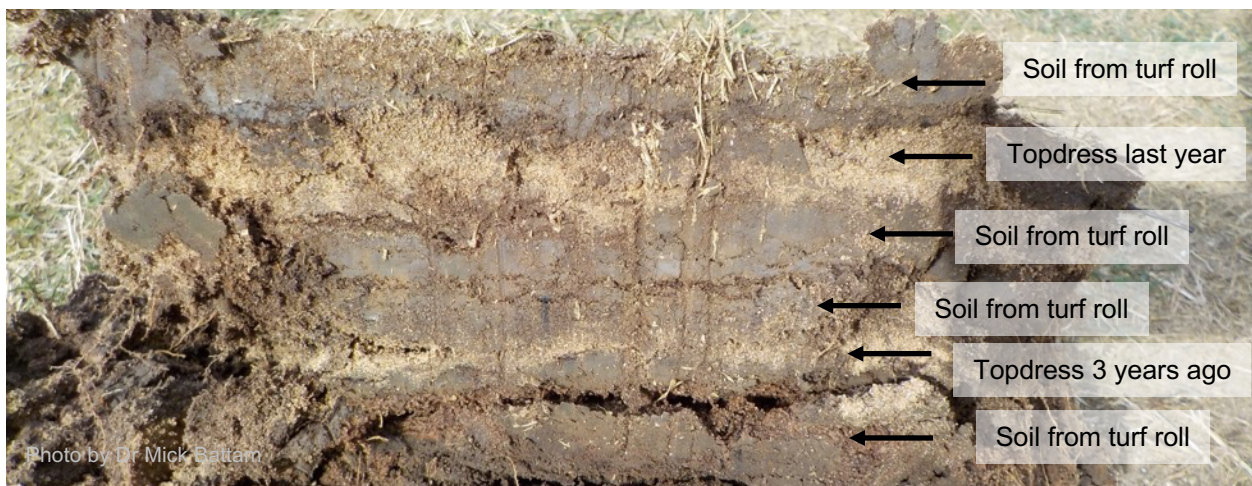
Figure 8.4: The soil profile on a site where turf patching of the same area is performed almost annually (upper). With all these layers, the water and roots struggle to penetrate into the profile. Amending the soil prior to patching resulted in these areas draining rapidly (lower).
