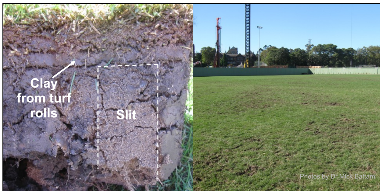
Figure 9.5: Turf with clay attached was laid over the top of slit drains (left), rendering the system almost completely useless so the field remained waterlogged (right).
