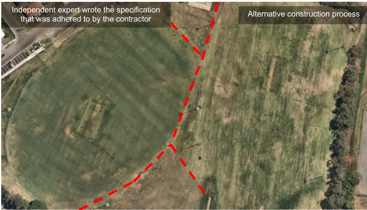
Figure E.3: Contrasting outcomes of two methodologies used to construct adjacent fields. The field on the left was rebuilt first according to best practice and performed above expectations. The field on the left has a superior playing surface, and 70% more carrying capacity during drought (Nearmaps image).
