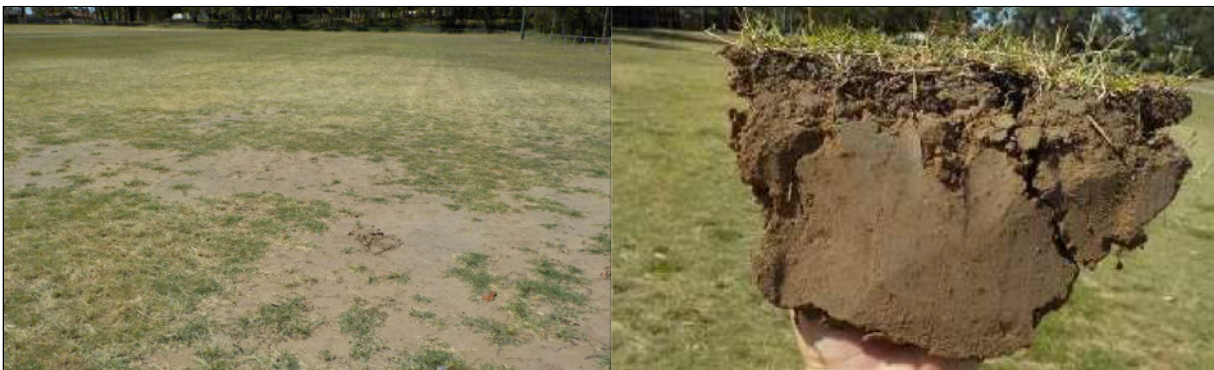
Figure 2.1: A third drop Clegg hammer reading of less than 120 is required for safe play on local sporting fields (Table 3.1). However, this field had readings ranging from 220 to 430, with the bitumen road having a value of 600. The incorporation of large quantities of organic matter is needed to address the hardsetting nature of many of the soils in the Lower Hunter. The reasons why soils in the Lower Hunter set hard are outlined in Book 2.
